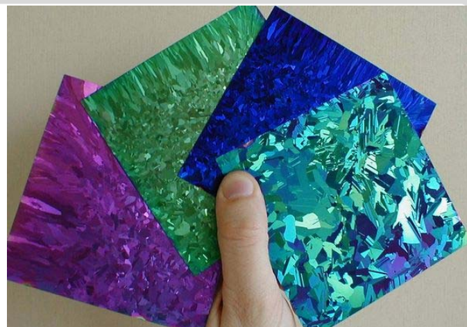
Four multocrystalline silicon (mc-Si) wafers covered with silicon nitride ARC
